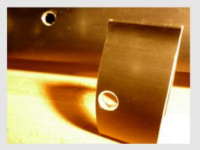
Look down the top of the mast, and feed one diamond wire up into the mast; twist the diamond wire until you can see that it is in line with the top bolt; then push the top bolt further into the mast and through the eye in the diamond wire (Photo 6).
