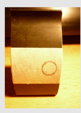
Mark the position of the diamond top bolt hole on both sides of the mast insert with a pencil (Photo 4).
